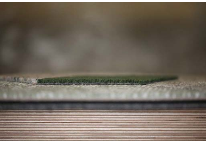
photo : section view with the different in height in the center of the tile (ca. 6mm higher for layer 1 + )
