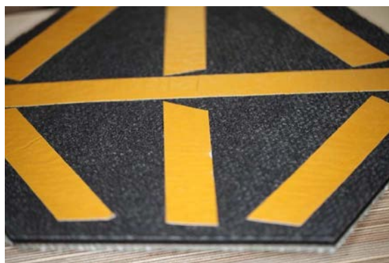
photo : backside of the wall tiles (the double-sided tape was not used for the mounting, the tiles were loosely laid on the floor of the reverberation room)
